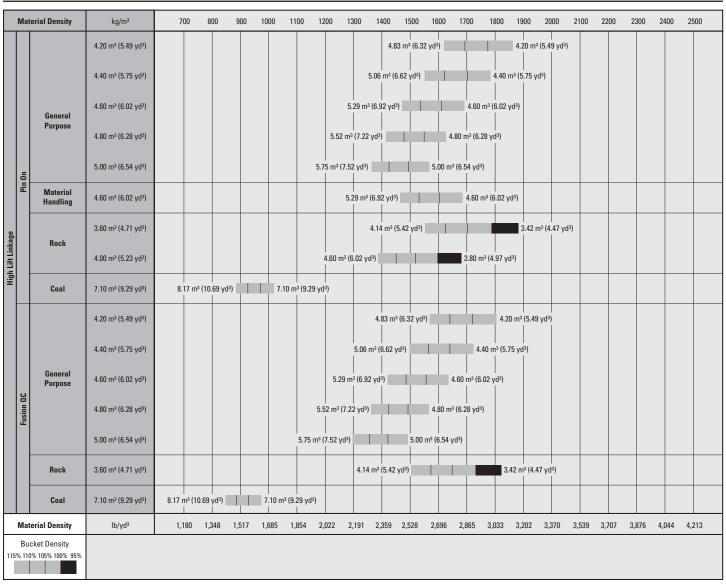
All buckets are showing Bolt-On Edges. Material Handling buckets are flat floor buckets.
