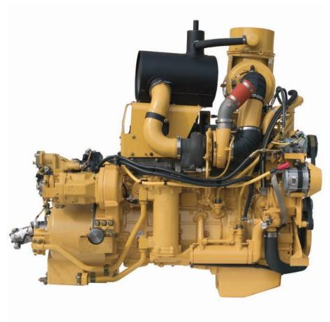
ATAAC and Turbocharging. Air-to-air aftercooling keeps air intake temperatures down and, in concert with the tight tolerance combustion chamber components, maximizes fuel efficiency and minimizes emissions. Significant improvements in air flow are generated by a water-cooled turbocharger, unique cross-flow head and single overhead cam.
