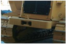
**Front Bumper.** A front bumper is mounted to the frame rails and provides both protection and a towing device. Pipelayer frame mounts are also an integral part of the frame.
