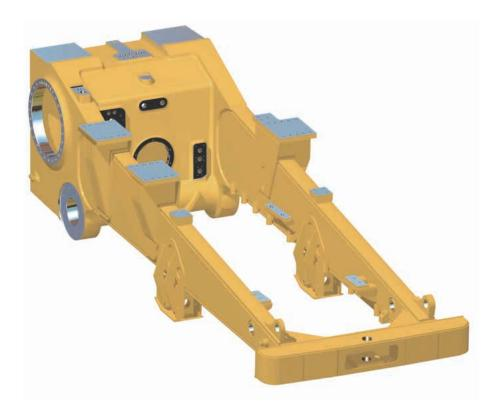
**Mainframe Strength.** The 587T mainframe is built to absorb high impact shock loads and twisting forces.
