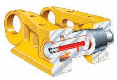
Positive Pin Retention (PPR) Sealed and Lubricated Track. Designed for high-impact and high load applications. The PPR exclusive Caterpillar design locks the link to the pin.
