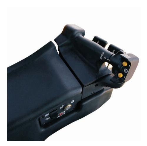
**Finger Tip Control (FTC).** Finger tip controls are clustered to the operator's left for easy one-handed operation, controlling steering, direction and gear selection.
