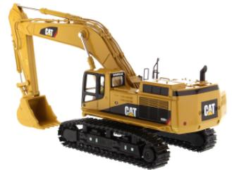
Still a favorite in any fleet, the Cat® 365B L Series II is at home in construction and demolition jobs, as well as mass excavation applications, quarries and mines. Powered by a Cat 3196 engine producing 404 hp (302 kw) this machine has the power and lift capacity to keep any operation running day after day.
