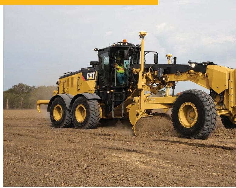
The front axle steering cylinder and sensing guards have been designed to enhance durability and hydraulic hoses have been routed to improve reliability.
