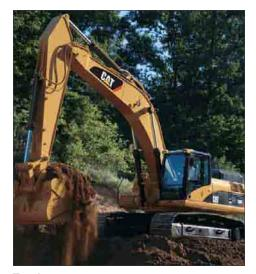
**Tracks.** The 336D comes standard with grease lubricated tracks. The track links are assembled and sealed with grease to decrease internal bushing wear, reduce travel noise and extend service life lowering operating costs.
