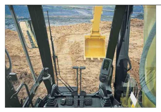
**Operator Station.** The workstation is spacious, quiet and comfortable, assuring high productivity during a long workday. The air conditioner and attachment switches are conveniently located on the right-hand wall, and the key switch and throttle dial are on the right-hand console. The monitor is easy to see and maximizes visibility.
