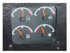
• **Gauge Cluster.** Maintains a constant display of vital machine functions, including: engine coolant temperature, hydraulic oil temperature, transmission oil temperature and fuel level.
