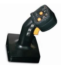
**STIC™ Steering Control.** STIC™ combines directional selection, gear selection and steering into a single lever for maximum responsiveness. Simple side-to-side motion turns machine right or left. Transmission shifting (forward/neutral/reverse) is controlled using a three position rocker switch. The thumb operated upshift and downshift button controls manual shifting.
