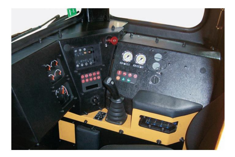
**Ergonomic Layout.** The operator station is ergonomically designed for total machine control in a comfortable, productive and safe environment. All controls, levers switches and gauges are positioned to maximize productivity and minimize operator fatigue.
