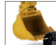
Moveable boom, stick and bucket
